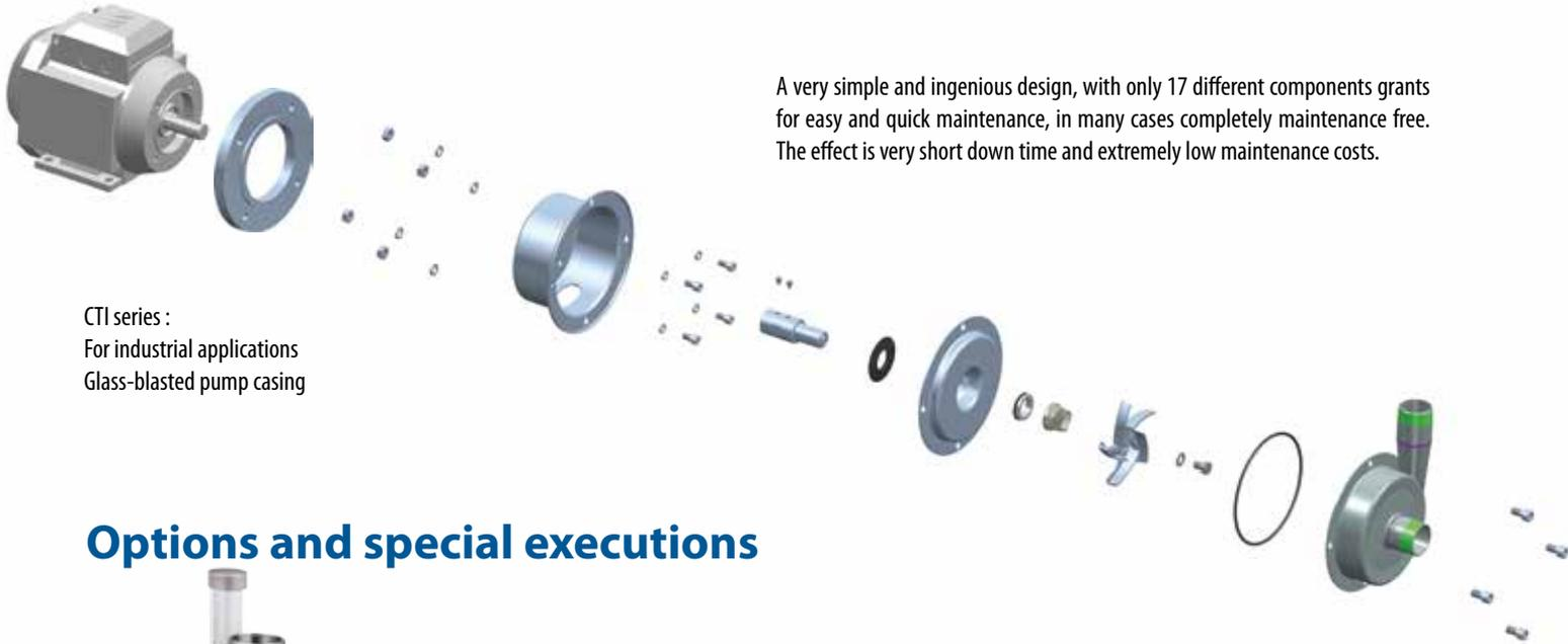
A very simple and ingenious design, with only 17 different components grants for easy and quick maintenance, in many cases completely maintenance free. The effect is very short down time and extremely low maintenance costs.
