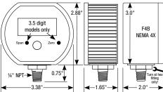
3.5 digit models use plastic caps on potentiometers, F4 covers are nylon screws with o-rings. 4 digit models use internal buttons.
