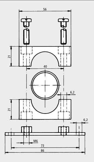
Width of the welding plates: 30 mm Thickness of the welding plates: 7 mm
