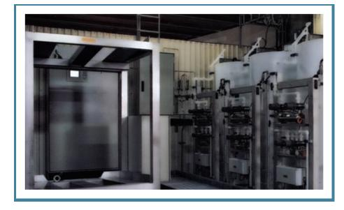
MEX<sup>™</sup> dilution system, providing precise dosage measurement and preparation of solution to desired concentration. The mixture is prepared in mixing tank (V=1100L), which also functions as a storage tank. The uniform quality of the diluted dye is controlled by dosing concentrated dye and water into a static pre-mixing vessel inside the tank, from which the diluted dye is conducted along an overflow pipe into the tank.
