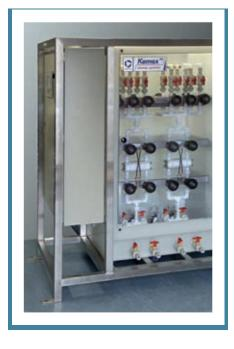
vel automation system (DCS) through binary signals (linespecific dosing control and alarm data) or via PROFIBUS fieldbus technology.
