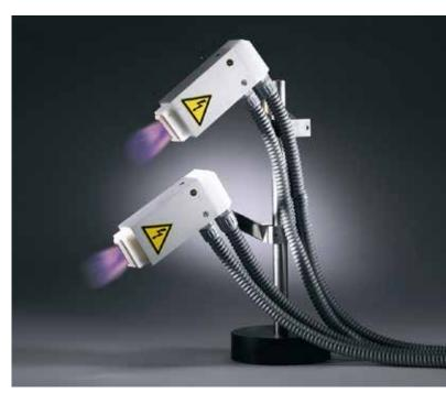
Tantec SpotTEC is used for treatment of profiles, cables and injection moulded parts. The SpotTEC is easily adapted into any production line and offers the user a high level of flexibility in use. The SpotTEC is based on the principle of high-voltage discharge in atmospheric air blown towards a substrate surface.
