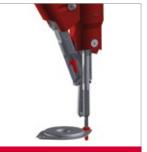
During the screwdriving process, the nose piece retracts upwardly away from the work piece without touching it
