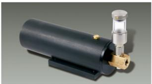
meets both of these requirements. Installed at the highest point of the hydraulic system, it completely vents the entire system after only a short time. Provided that there are no "air traps", the oil volume of the KOSTYRKA® air-oil hydraulic pressure intensifier can be used in its entirety.
