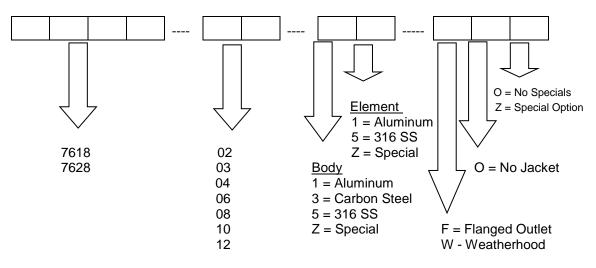
**EXAMPLE:** Model: 7618-04-11-F00 indicates a 4" Model 7618 with an Aluminum Body, and Aluminum Flame Element, Flanged inlet/outlet connections, and no special options.
