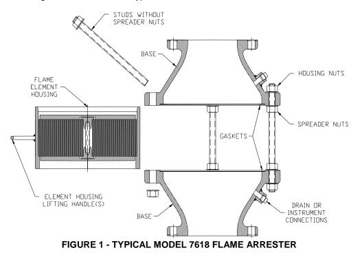
3. Loosen the housing nuts and remove only those studs necessary to withdraw the housing. Do not remove studs with spreader nuts.
