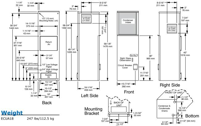
\*Condenser air outlet can be from either left or right side. Condenser air outlet can be selected in field.
