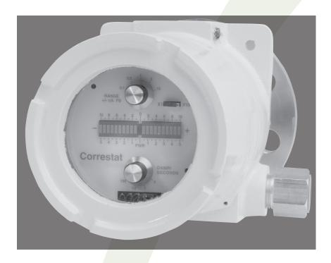
The Correstat 3430 electrostatic sensor monitors conditions within gas phase catalyst feed lines. It can monitor catalyst pulses and feeder changes, allowing plant operators to take appropriate action to avoid problems. With the real-time feedback from these electrostatic charge measurements, process continuity can be improved and shutdowns prevented.
