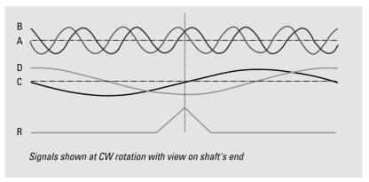
The incremental signals A and B and the zero signal R are differential voltage signals. The differential signal level is 1 Vpp. The zero signal appears once per revolution and reaches its maximum value at the angle where the amplitudes of A and B Signals are equal. The coarse tracks C and D deliver one sinewave period per revolution and are utilized to determine the absolute rotor position of Brushless DC motors for startup commutation. All signals have a DC offset of 2.5 V.
