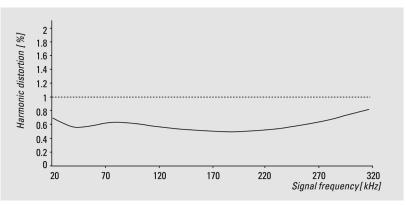
The quality of the servo loop is determined to a large extent by the absence of harmonics in the encoder's sinewave signals, particularly at low speed. In order to achieve high interpolation factors in the sequencing control, the incremental sinewave signals A and B are available with a harmonic distortion significantly under 1% throughout the specified temperature range. This delivers excellent synchronism and a high level of positional accuracy with servo axes.
