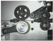
For rotational applications the Tru-Trac™ can be mounted in any orientation to monitor the position or velocity of many types of rotating equipment such as web tension control drums, rotary tables, printing, spooling, etc.
