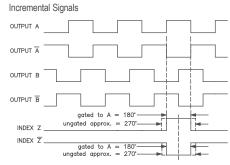
NOTE: ALL DEGREE REFERENCES ARE ELECTRICAL DEGREES ALL DEGREE REFERENCES ARE ELECTRICAL DEGREES. WAVEFORM SHOWN WITH OPTIONAL COMPLEMENTARY SIGNALS  $\bar{A}, \bar{B}, \bar{Z}$  FOR HV OUTPUT ONLY.
