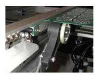
For linear applications the Tru-Trac<sup>™</sup> can be mounted above or below the moving object, and the tension on the wheel adjusted for a wide range of applications such as packaging, conveyors, mail sorting, cut to length, labeling, gantries, etc.
