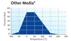
The temperature and pressure recommendations in the graphs apply to gaskets with a thickness of 2.0 mm and smooth flanges. Higher stresses are possible when thinner gaskets are used! \*Examplle for most common other media. Exact data for specific individual cases are available in the Frenzelit novaDISC programme or contact our application engineering specialists.
