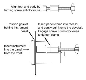
Fig 5 Fitting panel mounting clamps
