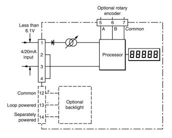
Fig 1 Simplified block diagram of BA427E
