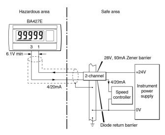
Fig 2 Typical application using barriers
