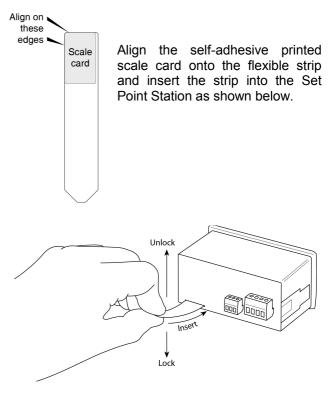
Fig 6 Inserting flexible strip carrying scale card into slot at the rear of Set Point Station.
