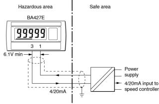
Fig 3 Typical application using a galvanic isolator
