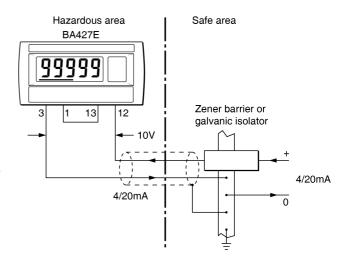
Fig 9 Loop powered backlight
