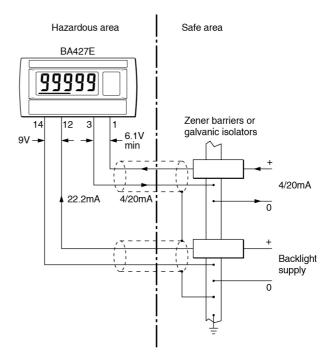
Fig 10 Separately powered backlight
