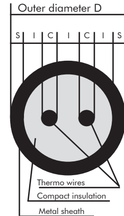
Cross-section of sheathed cable
