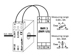
IMR 3 / IMR U3 measurement up to 60 A with IW 32  $\,$
