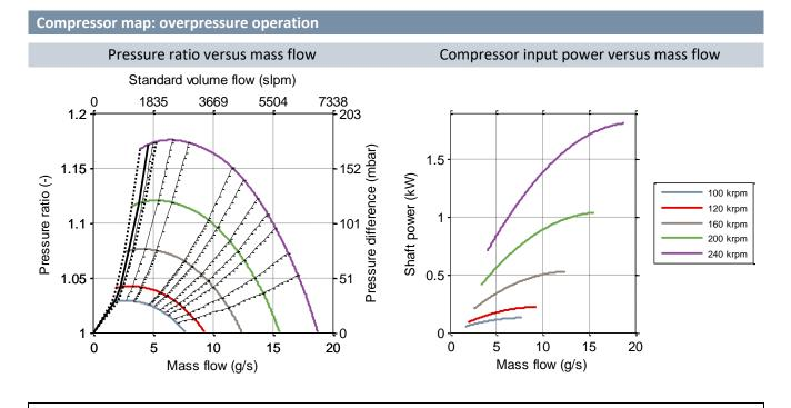
The specifications and compressor maps in this document for overpressure operation refer to helium at the inlet of the compressor: temperature:  $T = 293.15 K = 20^{\circ}C$ , absolute pressure:  $p_{in} = 1.013 bar abs$ .
