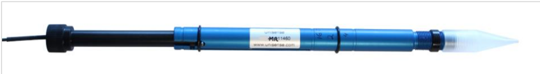
Figure 3: Microsensor mounted in the Microrespiration guide.
