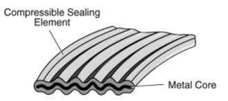
Klinger Maxigraph 104G has a lamination of 0.5 mm, I density, minimum purity 98 % graphite laminated to both sides, thus giving an initial soft seal enabling an effective seal to be obtained at low initial stress levels.
