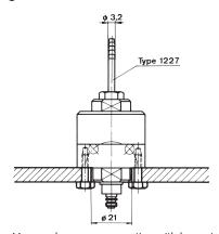
Fig. 2: Measured pressure connection with hose nipple
