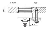
Fig. 4: Mounting with thread (left half) or flange (right half)
