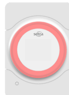
Red indicates alarm
