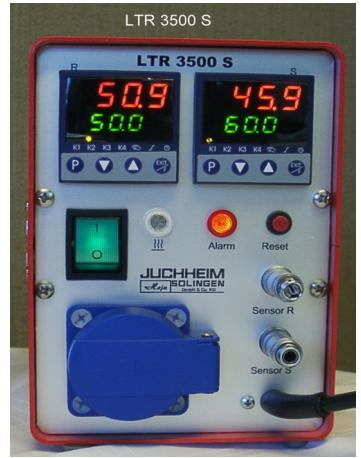
**Laboratory temperature controller LTR 3500 with microprocessor**
