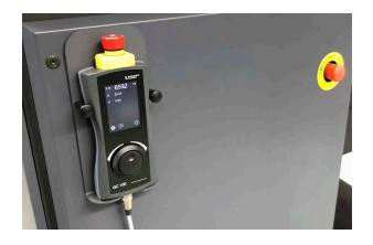
The stable metal holder attaches the GC 100 easily to the goniometer housing, the control rack or the laboratory wall.
