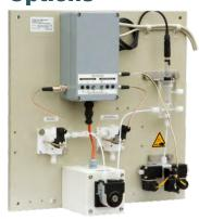
Acidifier/ Sparger/ Multiplexer-unit (ASM-unit; wall mounted)
