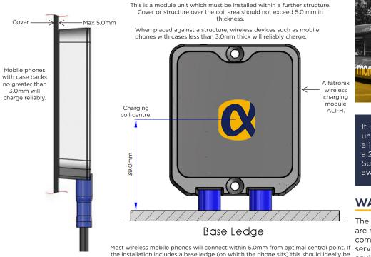
Most wireless mobile phones will connect within 5.0mm from optimal central point. If the installation includes a base ledge (on which the phone sits) this should ideally be placed 39.0mm from the centre of the ALI series module for optimum performance with a wide variety of mobile phones.
