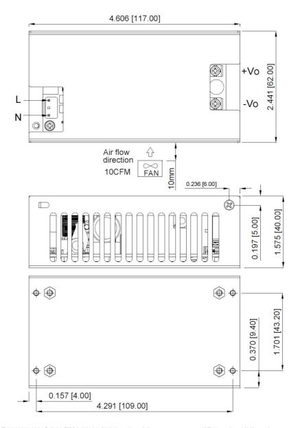
Input connector (L, N): TAIWAN KING PIN TERMINAL PVHI series. Mate connector: JST Housing VHR series or equivalent.
