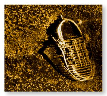
In the image above: The Burlington Horse Ferry, in Lake Champlain, VT. Image taken with Klein 4900 at 900Khz, 60m swath, 4knots, captured on the port side. Software: Klein SonarPro $^{\circ}$ .
