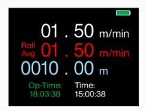
Available as a Standard or Advanced model, this portable, battery-powered monitor enables the pre-production setting and recording of travel speed rates for automated welding processes. It is capable of measuring welding time in seconds which provides valuable process costing data.
