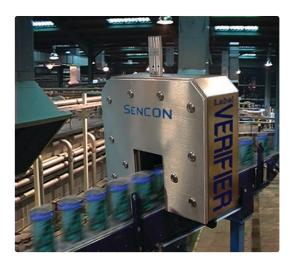
**MIXED LABELS** — The problem of "mixed labels" is caused by rogue cans left on the line after a batch changeover. Detecting and rejecting these cans without causing unnecessary spoilage is vital for reducing HFIs and avoiding customer complaint.
