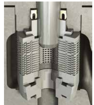
Class V metal seat with 500 PLI (pounds per linear inch of seating contact) loading force to achieve tight shut-off
