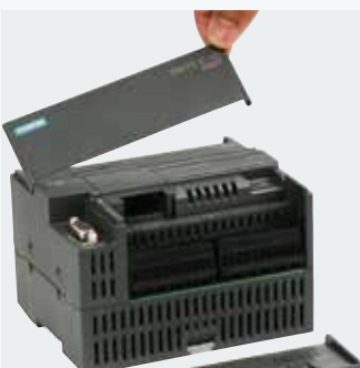
Remove the cover board of terminal
