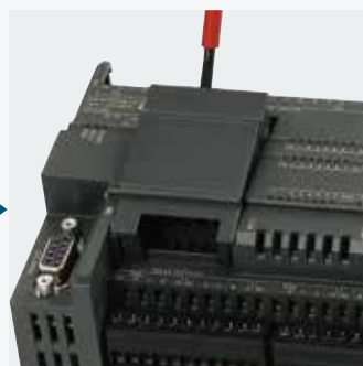
Remove the cover board with Screw driver
