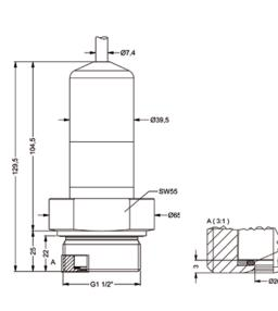
prepared for mounting with stainless steel pipe stainless steel / CuNiFe
