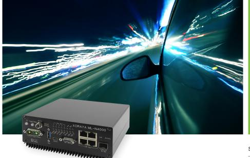
The XORAYA ML-N4000 is a compact and affordable automotive data logger capable of recording several bus systems simultaneously. Compared to its predecessor (XORAYA ML-Z7), it has significantly more powerful hardware, which records data with up to 4 Gbit/s. In addition, the logger is now equipped with an SFP+ interface (for 10GBase-T).
