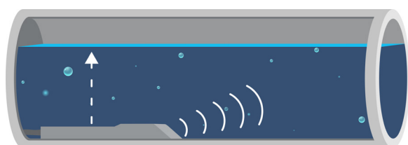
Submerged ultrasonic sensor measures level and velocity
