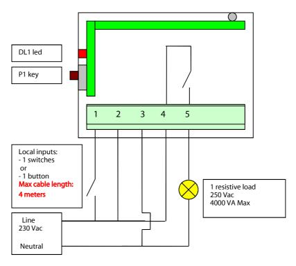
Schematic 1. Schematic indications for the control of one load
