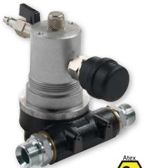
Pneumatic, selfpriming rotary vane pump for the transfer of petrol, with body in cast iron with anticorrosive coating and plastic rotor. On demand the pump can be supplied with an earth cable to enable an electrostatic discharge.
