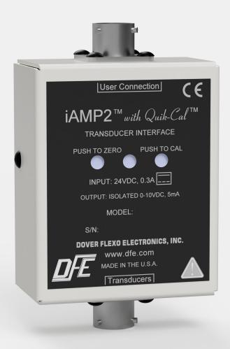
The iAMP2™ digital signal amplifier scales millivolt-level transducer (load cell) output to 0-10 VDC and 0-1 mA signals proportional to tension. The scaled output signals can interface with a drive, PLC, data logger or display meter.
