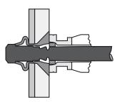
The Cherry patented shift washer collapses into itself, driving the locking collar into the head recess and into the stem locking groove to form an integral lock.
