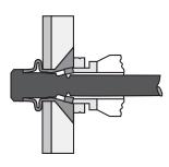
The stem is fractured at the break notch by continued pulling on the stem, thereby providing a flush, burr-free, installation.
