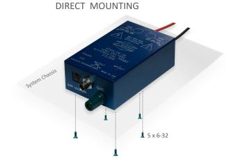
DP03 series probes can be mounted directly on a base plate or enclosure walls with 5 x 6-32 screws.
