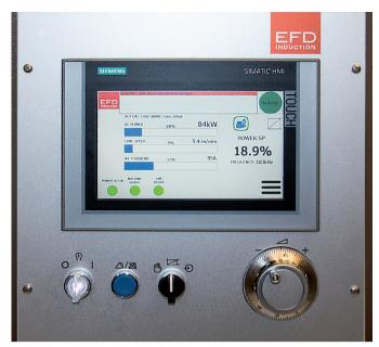
The Weldac is extremely easy to operate, with a minimum of manual settings. Operation is via an easy-to-use control panel.
