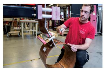
Coil changes take only seconds, with the frequency adjusting automatically to each tube dimension.
