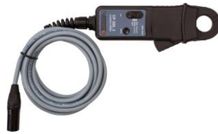
Current clamp 30/300 A power supplied from the instrument with extension 5 m (16.40 ft)
