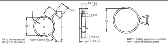
CTB Clamps should be installed/removed using the proper tool.
