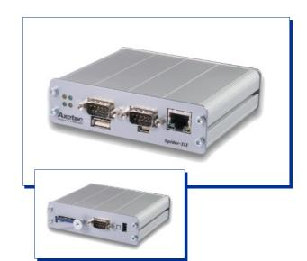
The Spider-III IX200 Embedded Linux computer supports 3 (optional 5) RS232 interfaces and a 10/100 Mbit Ethernet interface. Further available are a USB host, a USB device interface and a SD card slot for standard SD cards. The fanless IX200 has a very low power consumption and a robust design for a wide range of industrial applications.
