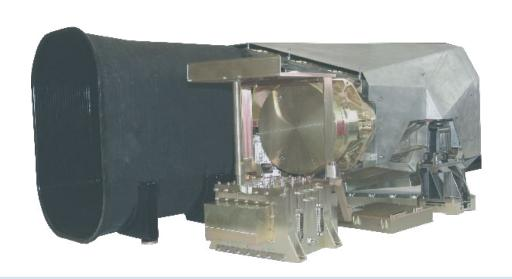
The JSS 56 is a compact, lightweight, long life and low cost multispectral imager product applicable to all professional small satellite platforms. Covering the Earth's surface continuously line-by-line (pushbroom principle) the imager of Jena-Optronik enables the precise data acquisition of an 77 kilometres wide strip of land with a pixel size of 6.5 metres out of 630 kilometres orbit height.
