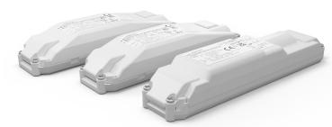
The eldoLED compact LED drivers are designed for downlighting applications in Europe and rest of world. The plastic housing is designed to fit through small cut-outs (down to 45mm) and includes a strain relief.
