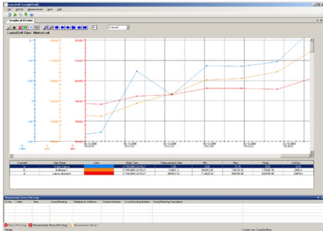
Fig. 1 The graphical window shows up to seven graphs. The user selects the data plotted, the scaling, and the style and color of the lines and background to build the graphical window.
