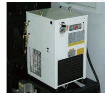
Spindle temperature control system (STD)
