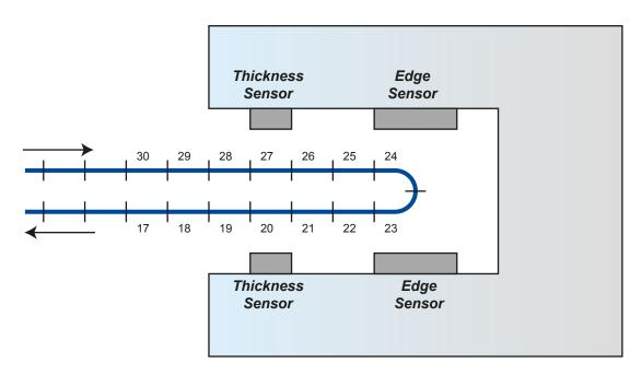
The complete film perimeter will be divided in several sections. The thickness sensor measures the sum of the upper and lower film sections. The rotating movement of the haul-off or the die causes a continuous variation of the measured sections.
