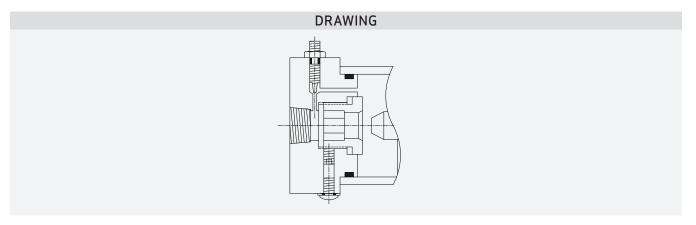
**Caution:** Cushion needles should be set between one half and one full turn from seated position. Setting should result in continuous speed reduction throughout the cushion length. Needle adjustment is set too far closed when there is an abrupt change in speed as the actuator enters the cushion. Never operate with needle in seated position or unscrewed beyond the point where the seal relief in the thread is visible.
