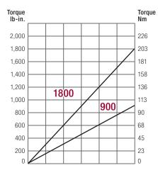
**TORQUE OUTPUT** VS. PRESSURE
