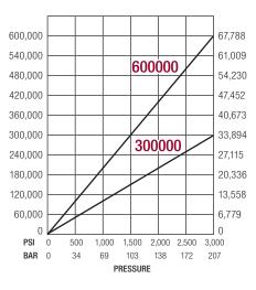
Output Torque (Ib-in.) @ Various Pressure\* Torque Model No.
