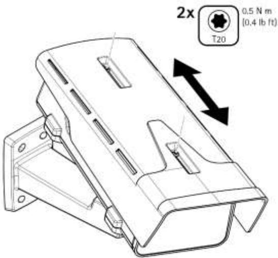
Adjust the weather shield: extend to the maximum without entering the field of view. This will protect the camera window from dirt and sideways disturbances by light sources to the maximum.
